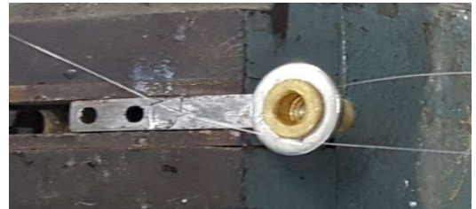
Fig. 4. FBGs bonded to the steel cantilever.
