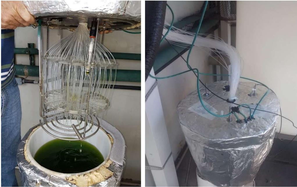
Figure 9. Left: Fiber arrangement inside de 30-liters PBR. The lower serpentine contains holes for aeration and CO<sub>2</sub> supply. The cylinder at top is the light sensor. Right: PBR closed, at the beginning of the cultivation. In both pictures it is possible to notice the thermal protection around the PBR to protect the cell culture against outside thermal oscillations.
