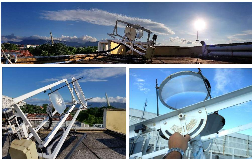
Figure 12. Upper: Solar tracker system installed on the roof of the Technology Center at the Universidade Federal do Rio de Janeiro. Bottom left: Details of the solar tracker, showing the stepper motor at center left, the microprocessor control box at bottom left, the Fresnel lens and the IR filter at the lens focus. Bottom right: Adjustment of the declination angle which allows the tracker to be directed to the sunrise direction.
