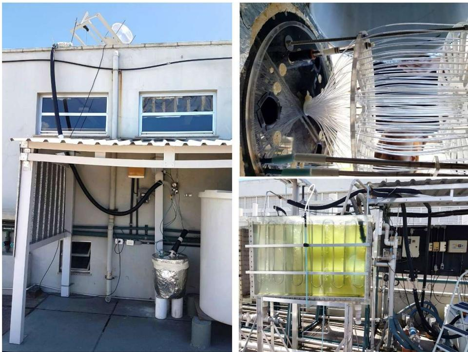
Figure 10. Left: Location of the PBR illuminated by the solar tracker at the roof of the building. The POF bundle connecting the PBR to the solar tracker is inside a black polyethylene jacket. Top-right: A detailed view of the POF arrangement inside the PBR. Lower-right: The conventional window PBR with its complex infrastructure, including a cold water pump and a refrigerator for temperature control.
