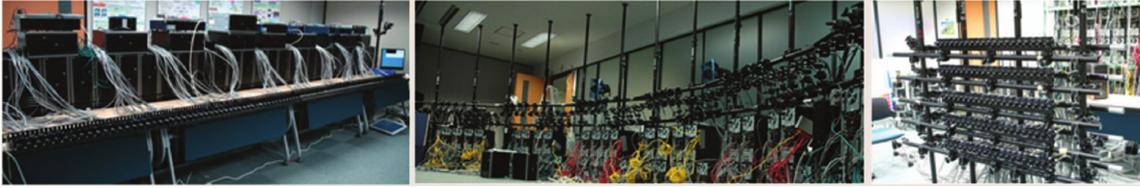
Figure 3.10: Three different arrangements for a 100-camera capturing system: linear (left), circular (centre) and 2D-array (right). Figure taken from [78].
