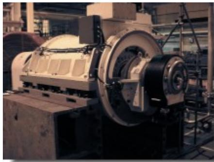
Fig. 7: Motor HTSAC (5 MW – 230 rpm).
